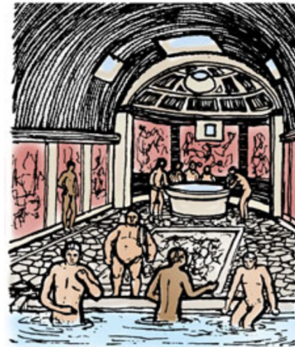
The caldarium (hot room) in the Forum Baths, Pompeii. At the nearer end note the large rectangular marble bath, which was filled with hot water. At the far end there is a stone basin for cold water. Rooms in baths often had grooved, curved ceilings to channel condensation down the walls.
