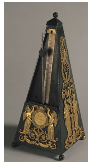
An early metronome owned by Beethoven; its inventor was a friend of his. A clock-work mechanism made the bar swing side to side, ticking at rates controlled by a movable weight.
