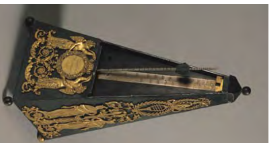
An early metronome owned by Beethoven; its inventor was a friend of his. A clockwork mechanism made the bar swing side to side, ticking at rates controlled by a movable weight.
