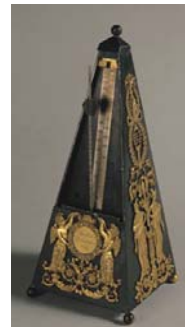
An early metronome owned by Beethoven; its inventor was a friend of his. A clockwork mechanism made the bar swing side to side, ticking at rates controlled by a movable weight.
